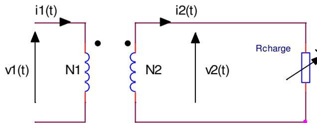
$$\eta = \frac{V_2.I_2.\cos \varphi_2}{V_2.I_2.\cos \varphi_2 + P_{fer} + R_s.I_2^2}$$
